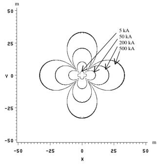
Figure 3: Horizontal view of positions at which nearby lightning flashes with peak currents of 5 kA, 50 kA, 200 kA and 500 kA can trigger the lightning sensor system with two loop antennae placed on opposite sides of a wind turbine with tower radius 1 m. The vertical axis of the tower is at (x,y)=(0,0) and the plane of the loop antennae are parallel to the x-axis.
