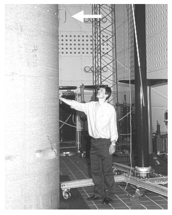
Figure 4: Laboratory testing of the sensor system. The loop antennae were mounted at a height of 3 m on opposite sides of a eight m high wind turbine tower section.
