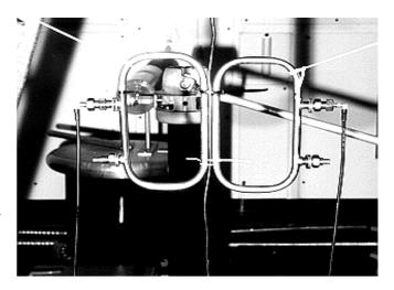
Figure 5: Scale test where the two loop antennae are brought closer together and subjected to a magnetic field corresponding to that of lightning flashes with high peak lightning current levels.
