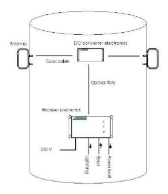
Figure 1: System overview showing the two loop antennae placed on opposite sides of the tower , the cabling and the electronics boxes – drawing not to scale.
