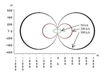
Figure 2: Horizontal view of positions at which nearby lightning with peak currents of 50 kA, 200 kA and 500 kA can trigger a lightning sensor system with only one loop antenna placed on the side of a wind turbine with tower radius 1 m. The vertical axis of the tower is at (x,y)=(0,0) and the plane of the loop antenna is parallel to the x-axis.
